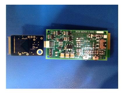
RCB-LVDS Module connected to Intan amplifier board using 1m blue cable.
