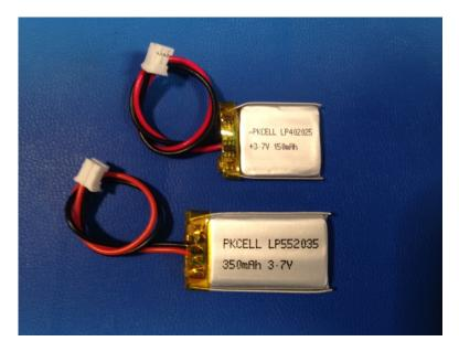
Battery capacity will determine the standby and streaming time you can achieve before needing to recharge.
