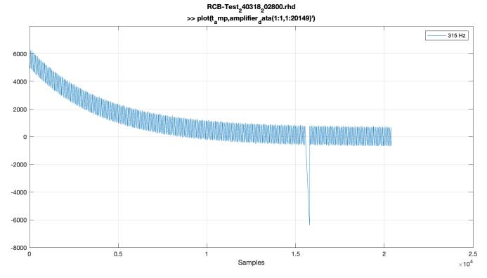
Recording shows data samples from start of a session. The initial values show data before the RHD on-chip dc removal filter settles out. When channels = 32, there will be 21 samples for each channel in each UDP packet. Since the first UDP data packet is always discarded t\_amp index starts at 21.
