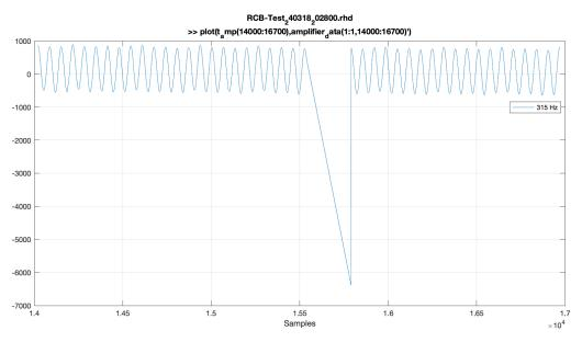
Looking at t\_amp we see 12 repeat timestamps. These correspond to the 12 lost UDP data packets. When channels = 32, there will be 21 samples per channel in each UDP packet.
