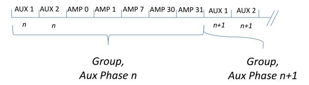
Fig. 3. Illustration of data, sequence of groups for auxMask = 6, chanMask = 0xC0000083. The group consists of 7 words, or 14 bytes.
