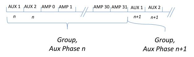
Fig. 2. Illustration of data, sequence of groups for auxMask = 6, chanMask = 0xFFFFFFFF. The group consists of 34 words, or 68 bytes.
